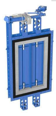
Flanged light butterfly, square, rectangular louvred type, several blades.. Welded construction body and disc. Manufactured with different kinds of tightness depending the customer requirements (100% tight, 99,5% tight o 98,5% tight). Fabrication materials: S275JR carbon steel, HII carbon steel, 16MO3 carbon steel, different stainless steel qualities (aisi 304, 316, 310 ...).
